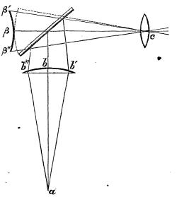
to receive centrically the reflected diverging pencil from the bubble will cause it to emerge in a parallel pencil, thus placing the image at an infinite distance, and enabling us to view it through a telescope.
